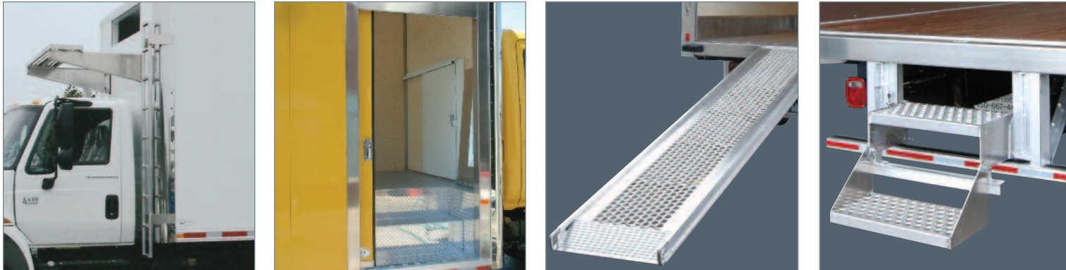
Exterior ladder for refrigeration unit access
